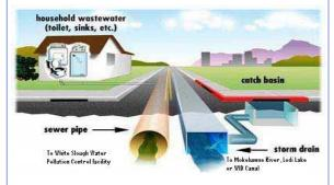
The Sanitary Sewer System collects wastewater from indoor plumbing such as sinks, toilets, washing machines, and floor drains where it is transported through underground pipes to a sewage treatment plant. The treatment plant removes many pollutants from wastewater before it is discharged back into a river.
